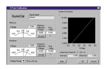
5. Set the bellows so that the scale reads 0 liters. Click the Accept button for the Minimum Calibration voltage.
