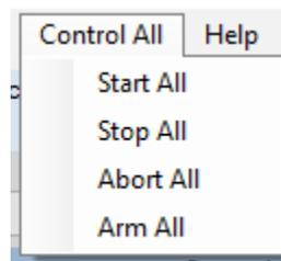
The Control All menu provides controls for starting, stopping, and aborting all channels.
