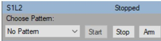
Start - Starts playback of the pattern. This control is only enabled when the channel has a pattern selected and is armed.
