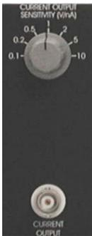
The CURRENT OUTPUT unit consists of (6) CURRENT OUTPUT SENSITIVITY V/nA switch and (29) CURRENT OUTPUT connector.
