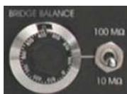
The BRIDGE BALANCE unit consists of (20) 100 MΩ / 10 MΩ RANGE switch and (21) BRIDGE BALANCE potentiometer.
